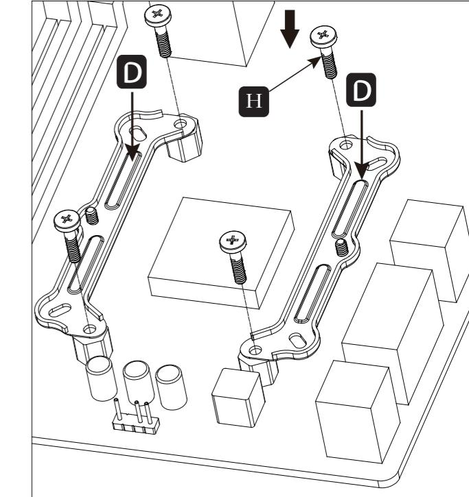
Install the mounting brackets and secure with screw
