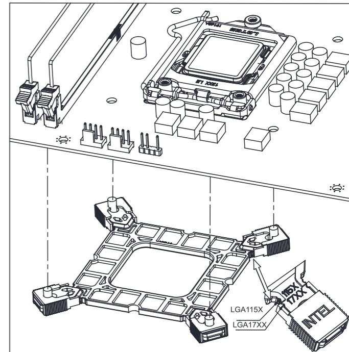
Install the backplate to the motherboard and fix it with spacers
