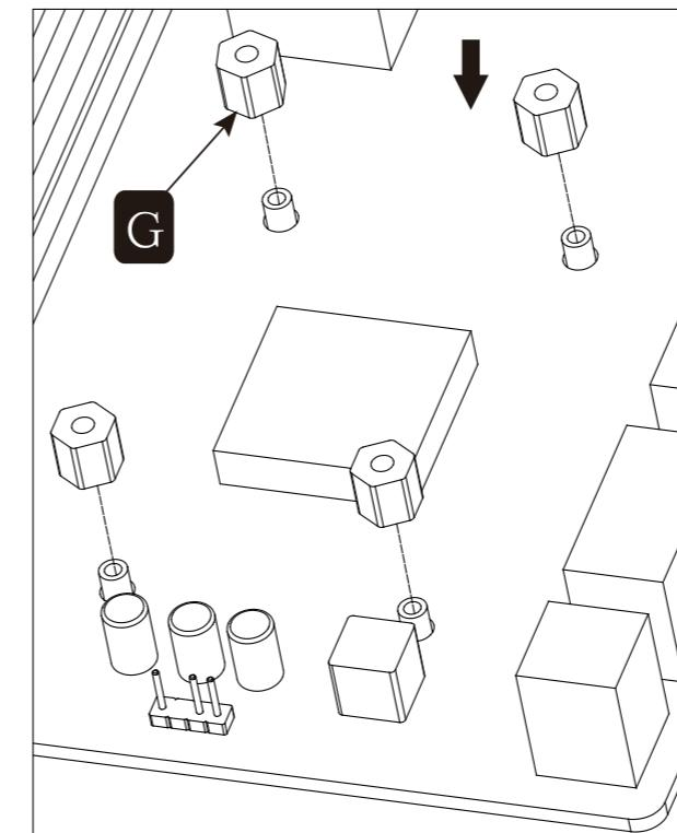
Installation of AMD spacer column
